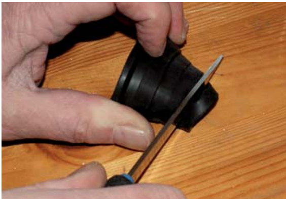
7. For 25 mm Pipe-in-Pipe, use the pre-cut LK Housing Pipe Bush 25 (Art. no. 187 44 83). NOTE: These items are ordered separately.
