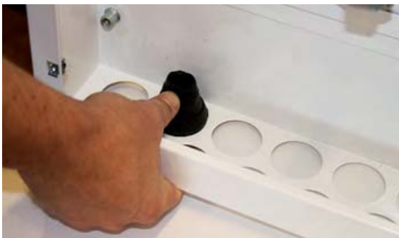
8. The pipe inlet is pushed into the hole so that it tightens properly. Ensure that no components e.g. wall studs or discs are pressed against the cabinet grommets, as this may cause leakage.
