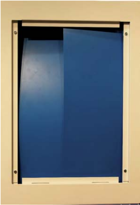
16. Assemble the splashguards. These should be assembled during the construction to prevent dirt and dust from getting in to the cabinet.
