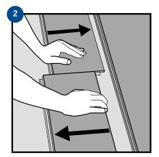
Disassemble the panels by sliding horisontally. (Do not fold up.)
