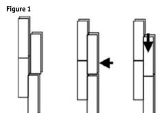
\* Ultraloc with transverse rib middle layer: First tap together the short end and then the long side, starting with the free end. (fig. 2)
