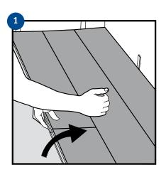
Separate the whole row by carefully lifting up and slightly knocking just above the joint. Fold up and release the whole longside.
