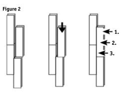
2-lock are angled locking systems, with the boards joined by angling in and pressing down into the profile of the previous board.
